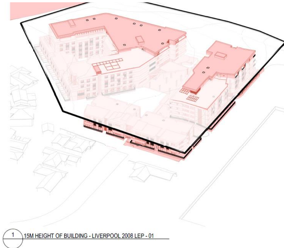
Figure 21: 3D view from Randwick Close frontage of Buildings A on left and Building B on right showing portion of buildings which projects through the 15m HOB control Source: Jackson Teece Drawing DA852B
