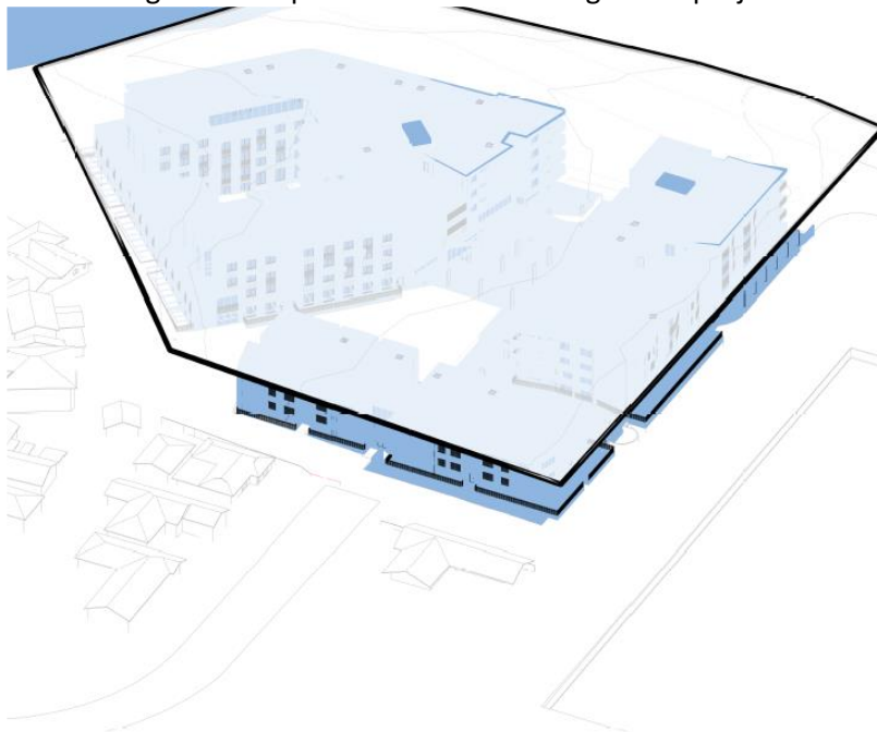
Figure 23: 3D view from Randwick Close frontage of Buildings A on left and Building B on right showing portion of buildings which projects through 18m Source: Jackson Teece Drawing DA852B
